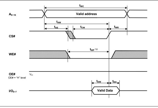
Note 22.  $t_{WP}$  is the interval between write start and write end.
